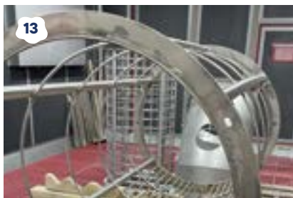
13 Stainless steel surfaces get glass bead blasted
