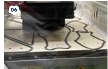
HPL panels are precisely shaped using CNC milling technology
