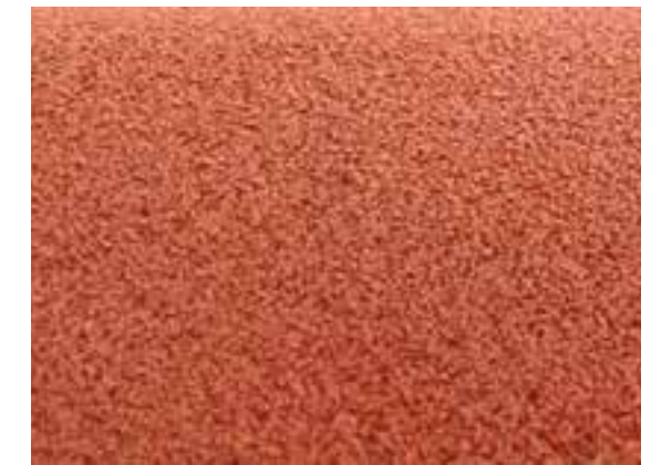
Platform surfacing: 4mm pre pressed EPDM mat
